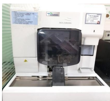
Figure 1: Five part fully automated haematological analyser Sysmex-XT 1800-i
