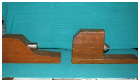
Picture 4: Insertion of specimen into tooth space in resin filled with polyvinyl siloxane
