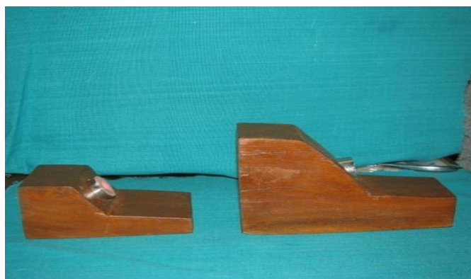
Picture 3: Blocks prepared to receive cylinders for angles 70° and 45°.
