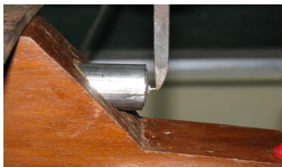
Picture 6: Failure of Fiber post specimen
