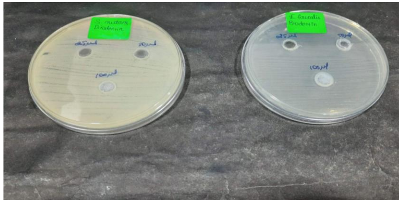
Fig 1: Agar diffusion plates containing S. mutans and E. faecalis with different concentrations of Biodentine.
