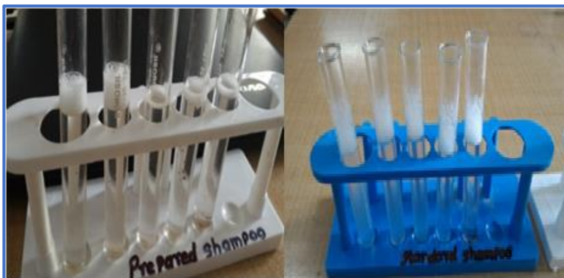
Figure No. 3: Foaming ability and foaming stability test of prepared and standard shampoo.
