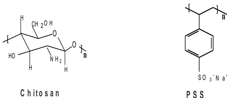
**Figure 1:** Polyelectrolytes used for coating
