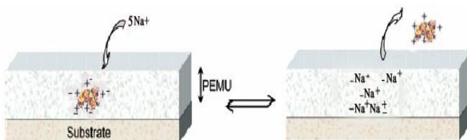
**Figure 4:** Displacement of loaded proteins from the multilayer, where salt counter ions replace adsorbed proteins in high salt concentration.
